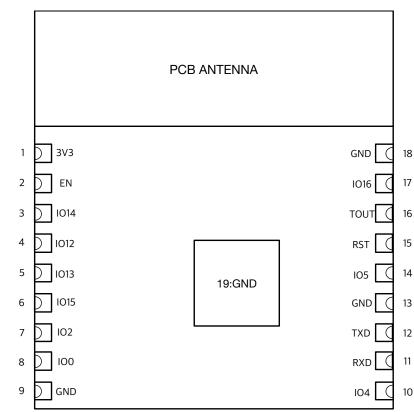
Figure 2-1 shows the pin distribution of the ESP-WROOM-02.
