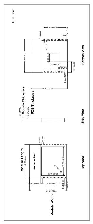
Figure 6-1. Dimensions of ESP-WROOM-02
