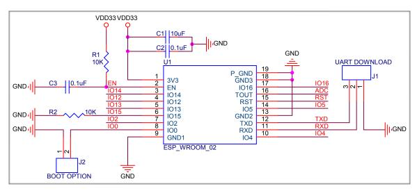
Figure 5-2. ESP-WROOM-02 Peripheral Schematics
