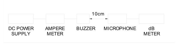
In the measuring test, buzzer is placed as follows:
