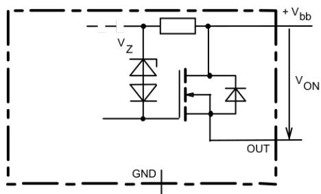
$V_{ON}$  clamped to 58 V typ.
