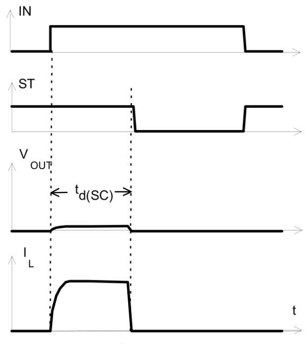
$t_{d(SC)}$  approx. 200  $\mu\text{s}$  if  $V_{bb} - V_{OUT} > 8.3 \text{ V typ.}$
