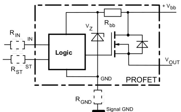
$R_{bb} = 120 \Omega$  typ.,  $V_Z + R_{bb} * 40 \text{ mA} = 67$  V typ., add  $R_{GND}$ ,  $R_{IN}$ ,  $R_{ST}$  for extended protection
