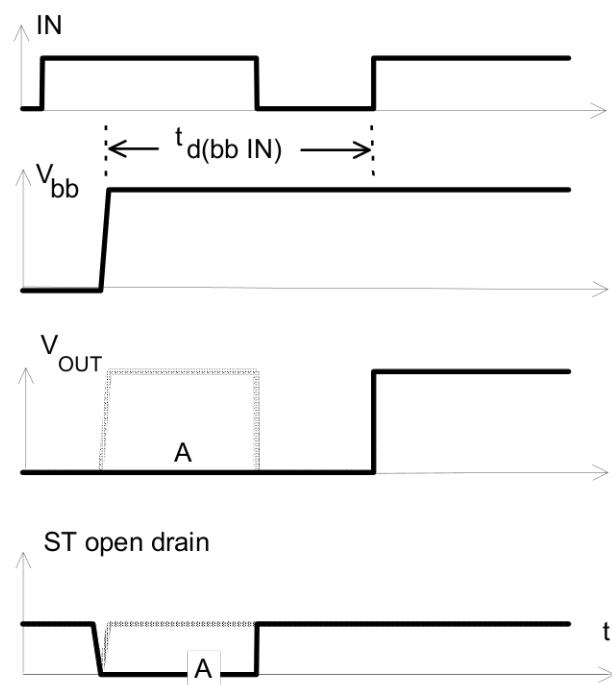
in case of too early  $V_{IN}=\text{high}$  the device may not turn on (curve A)
