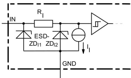
ZD<sub>I1</sub> 6.1 V typ., ESD zener diodes are not designed for continuous current
