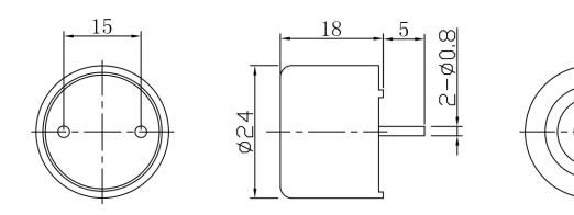
Housing material: ABS Wave solder and wash not allowed.
