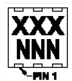
6-Lead DFN (2x2x0.9 mm)
