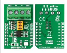
RS485 Click 3.3V is an accessory board in mikroBus<sup>TM</sup> form factor. The on-board SN65HVD12 differential line transceiver is suitable for high speed bidirectional data communication on multipoint bus transmission lines. It is designed for balanced data transmission and complies with EIA RS-485 standard. This transceiver features a differential line driver and differential line receiver. Board is set to use 3.3V power supply only.
