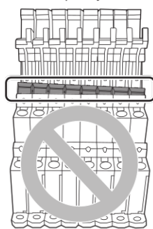
Incorrect installation Some terminals not inserted completely.
