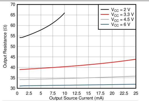
Figure 2. Output driver resistance in High state
