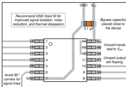
Figure 11. Example layout for the SN74HCS7002
