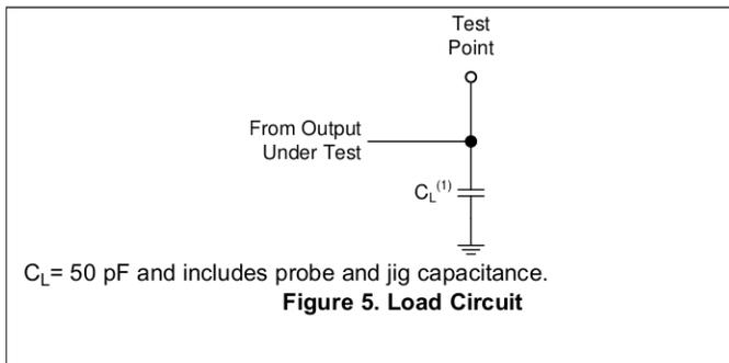
Figure 5. Load Circuit
