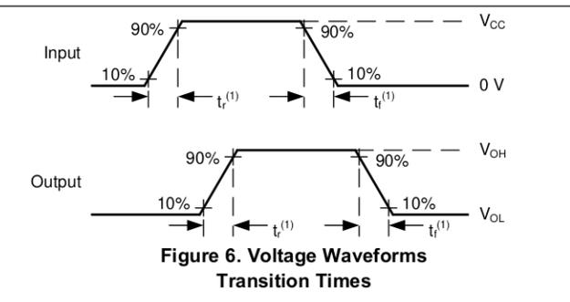
Figure 6. Voltage Waveforms Transition Times
