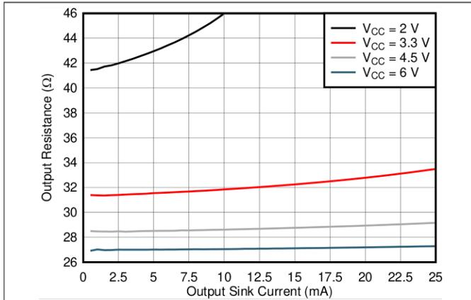
Figure 1. Output driver resistance in Low state
