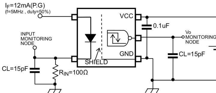
CL is capacitance of the probe and JIG.
