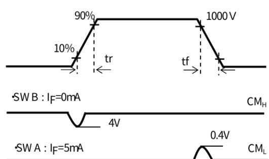
$$CM_H = \frac{800(V)}{t_r(\mu s)} \quad CM_L = \frac{800(V)}{t_f(\mu s)}$$
