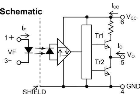
0.1uF bypass capacitor must be connected between pins 6 and 4
