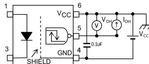
TEST CIRCUIT 3 :  $I_{CCL}$
