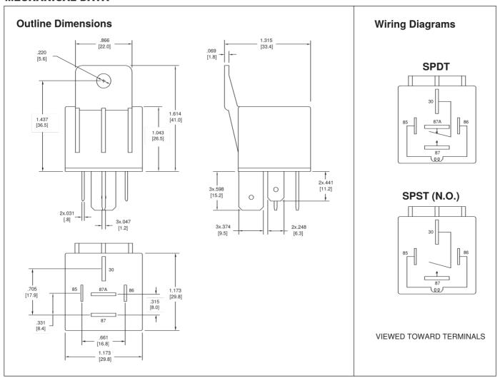
Dimensions in inches with metric equivalents in parentheses. Tolerance: ± .010"
